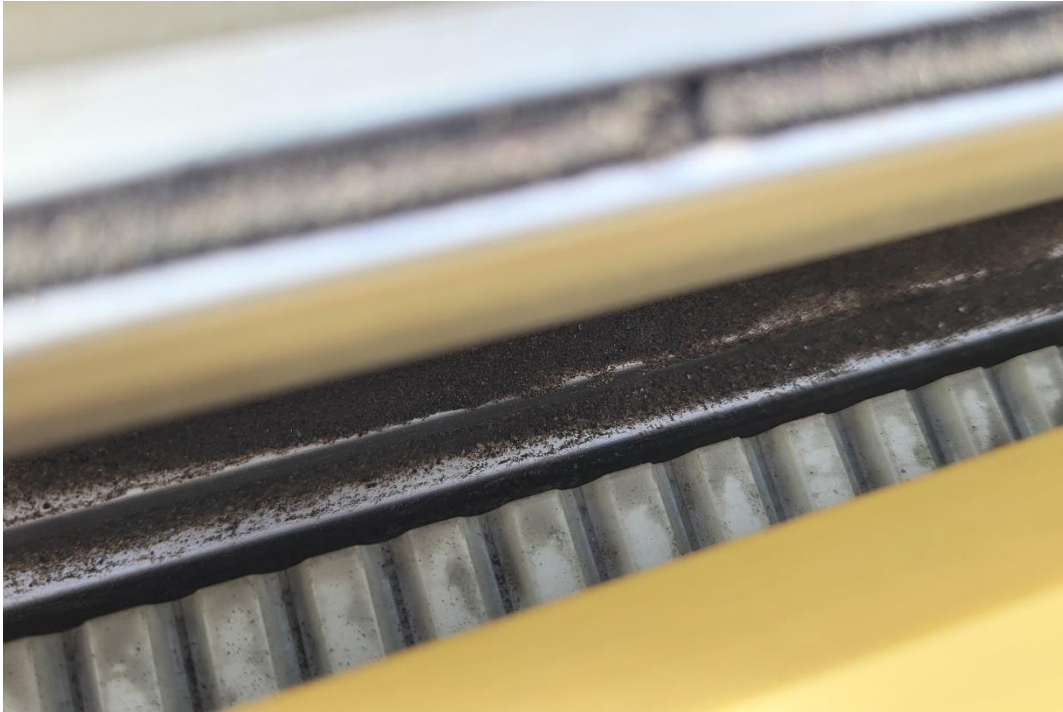
Photo 3-2 Grit Accumulation on Trolley Guide Surfaces within Traversing Beam
